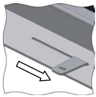
Fig. 33: Combustion air slider
