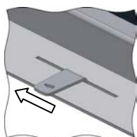
Fig. 27: Combustion air slider
