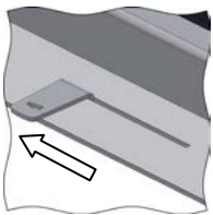
Fig. 38: Combustion air slider
