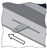
Fig. 34: Combustion air slider
