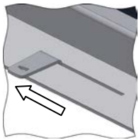
Fig. 45: Combustion air slider
