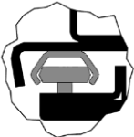
Fig. 62: C-shaped rail and guide rollers
